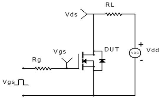
Figure 2: Resistive Switching Test Circuit & Waveform
