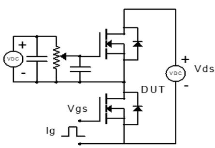
Figure 1: Gate Charge Test Circuit & Waveform
