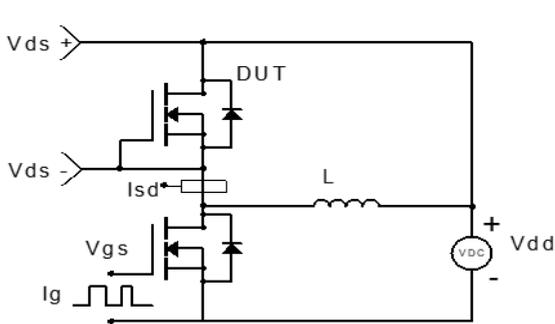
Figure 4: Diode Recovery Test Circuit & Waveform
