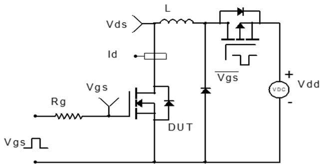
Figure 3: Unclamped Inductive Switching Test Circuit & Waveform
