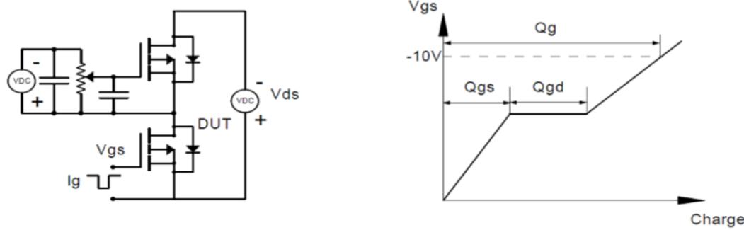
**Figure 1: Gate Charge Test Circuit & Waveform**
