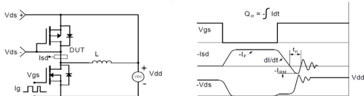
**Figure 4: Diode Recovery Test Circuit & Waveform**
