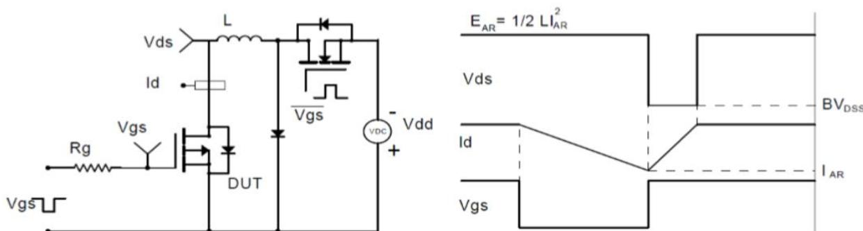
**Figure 3: Unclamped Inductive Switching Test Circuit & Waveform**
